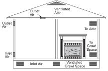
Figure 4 - Ventilation Air from Outdoors
